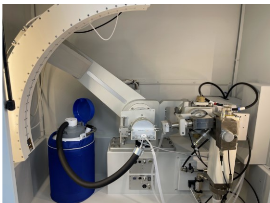
X-ray/XRD Temperature stage with ThermoFisher X-Ray diffraction system
