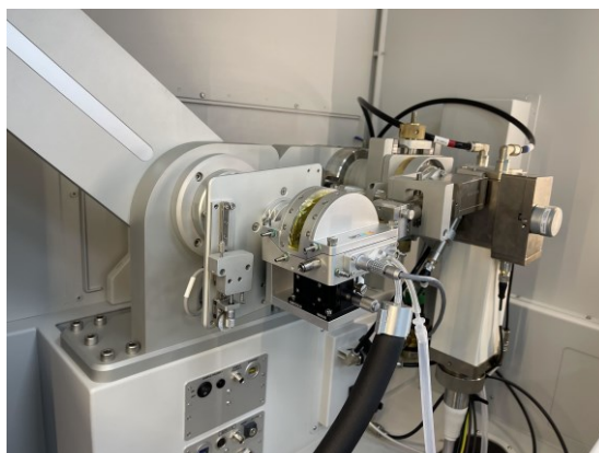
X-ray/XRD Temperature stage with ThermoFisher X-Ray diffraction system
