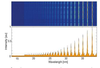
Sample measurement demonstrating the resolving power of maxLIGHT. The shown high harmonic spectrum is generated by the interaction of a single femtosecond laser pulse with a solid target and subsequent spectral filtering. The substructure inherent to the generation process is clearly resolved by the XUV spectrometer.
