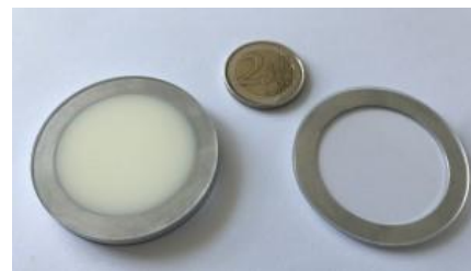
Cuvette of the SphereSpectro 150H system with special shape and small dimensions for direct attachment on the measurement port
